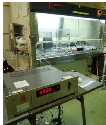
Left: Exposure to ozone within the box; Right: Concentration control using an ozone concentration monitor
